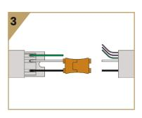
3. Complete wire make up inside housing using wire nuts supplied by Artience Lighting. If remote driver housing is located in an attic, CL3 cable must be used to connect power from the driver to the fixture.
