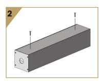
2. Secure the housing to the surface using fasteners (provided by others). Remote driver housings must be spaced at least 3" apart.
