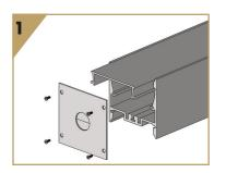
1. Remove one end of the housing by removing the four screws securing the end cap, and slide out the lid.
