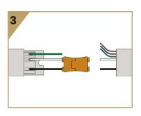
3. Complete wire make up inside housing using wire nuts supplied by Artience Lighting. If remote driver housing is located in an attic, CL3 cable must be used to connect power from the driver to the fixture. Ground the LED driver inside the driver box as well with grounding from the building.
