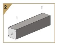
2. Secure the housing to the surface with supplied fasteners. Remote driver housings must be spaced at least 3" apart.
