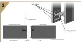
Insert Light Leak Gasket into the extrusion as indicated in illustration number 3. Note that the gasket will extend past the extrusion.
