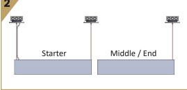
3. Thread Aircraft Cable of Middle Fixture through Canopy Mounting Nut and Canopy, then follow the NON Power SIDE instructions above. If a Power Cord is indicated, follow the Power FEED SIDE instructions above.
