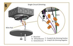
5. Secure Canopy to the Bracket Bar by fasting the Canopy Mounting Nut to the Cable Gripper.
