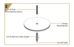
3. If using a J-Box and 3-0 Mud Ring: Install Bracket Bar to J-Box (provided by others) with (2) 8-32 Bracket Bar Screws, and install Cable Gripper. Thread Aircraft Cable through Canopy Mounting Nut and Canopy before inserting into Cable Gripper. Attach Bell Crimp before using level to adjust to desired height. Secure Canopy to the Bracket Bar by fasting the Canopy Mounting Nut to the Cable Gripper.
