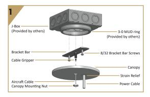
Install Bracket Bar to J-Box (provided by others) with (2) 8-32 Bracket Bar Screws, and install the Cable Gripper into the Bracket Bar.
