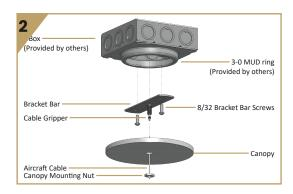
2. Thread the Aircraft Cable through the Canopy Mounting Nut and the Canopy before inserting the Cable into the Cable Gripper.
