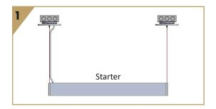
1. Install Starter fixture using the same steps used to install an individual fixture.
