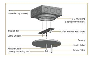
1. Install Bracket Bar to J-Box (provided by others) with (2) 8-32 Bracket Bar Screws, and install the Cable Gripper into the Bracket Bar.
