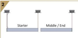
2. Remove the LED Tray and Lens of Middle fixture (the next fixture in the run) and carefully set aside. Touching LEDs can damage them and result in a voided warranty.
