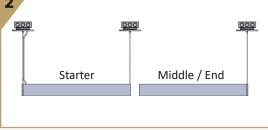
3. Thread Aircraft Cable of Middle Fixture through Canopy Mounting Nut and Canopy, then follow the NON Power SIDE instructions above. If a Power Cord is indicated, follow the Power FEED SIDE instructions above.
