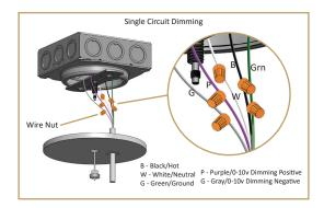
4. Connect the Power Cord to the existing wires in the J-Box, completing the wire makeup by following all national and local electrical laws and codes.
