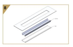
8. Carefully replace the LED tray, connecting the BLUE and RED wires to the corresponding port on the driver. **TOUCHING LEDs CAN DAMAGE THEM AND RESULT IN A VOIDED WARRANTY.**
