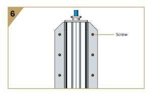
6. Stagger screws and keep spacing to a maximum of 5".
