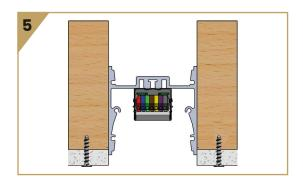
5. Fit fixture into roughed opening and secure with drywall screws (provided by others).
